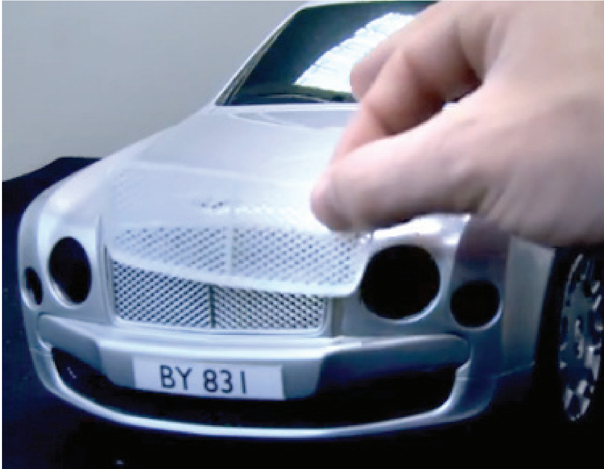
Bentley Motors designers print miniature scale models of vehicle interiors and exteriors.
